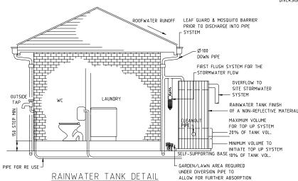
FIRST FLUSH OF CONTAMINATED WATER IS DIVERTED INTO CHAMBER WATER FLOW SLOW RELEASE OF STORMWATER AFTER STORM EVENT.
