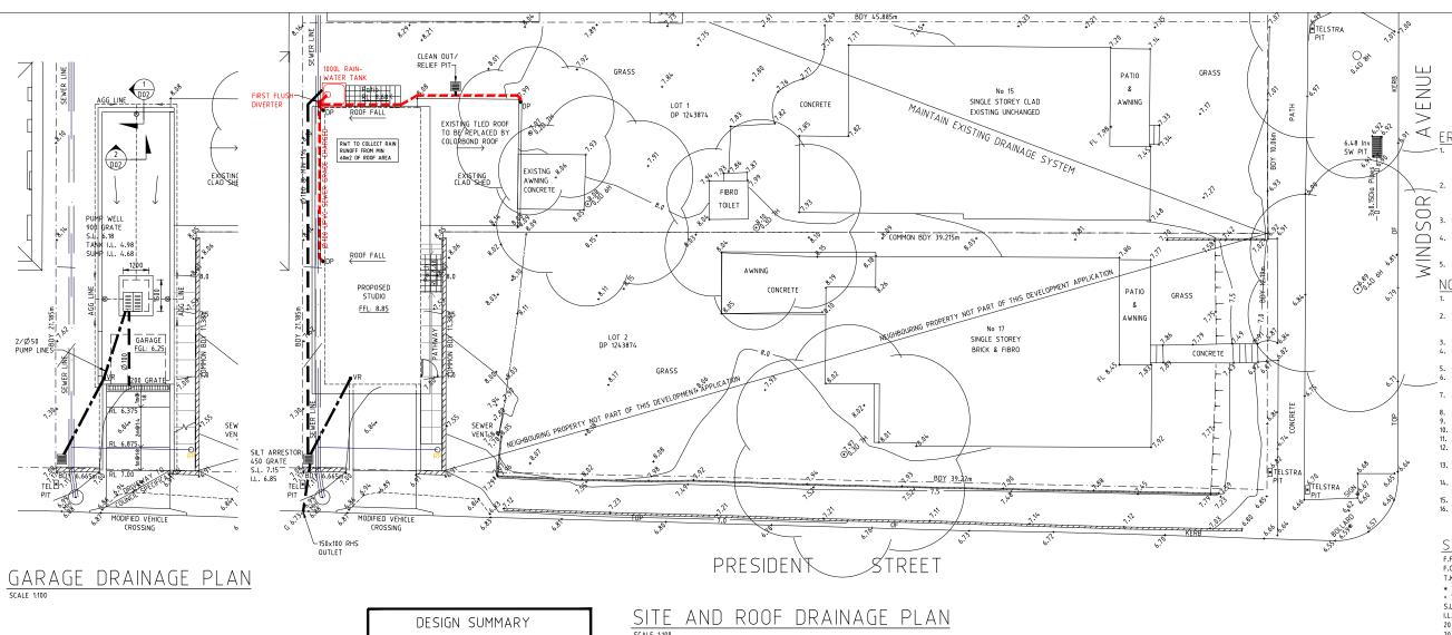
TOTAL SITE AREA = 537m2 PRE DEV. IMP. AREA = 208m2 (39%) POST DEV. IMP. AREA = 318m2 (59%) PROPOSED IMPERVIOUS AREA IS LESS THAN 70%, THEREFORE NO O.S.D. IS REQUIRED. IN ACCORDANCE WITH CANTERBURY DCP 2012. SECTION B5.5
